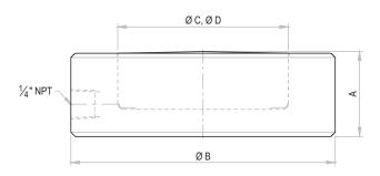
OLPVL Series - O Orione L Single acting Load return P Plain ram VL Very Low height 10 Capacity - ton 10 Stroke - mm
